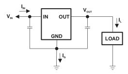
$$\begin{split} I_I &= I_L + I_G \\ P_D &= (V_{IN} - V_{OUT})I_L + (V_{IN})I_G \end{split}$$
